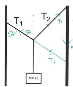
The diagram on the left shows a box of mass 100.0kg suspended by two cables. T1 is attached to a vertical wall at angle of 54.0°, while T2 is attached to another vertical wall at angle of 31.0°.
