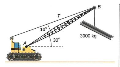
A 12.0m boom, AB, of a crane supporting a  $3.00 \times 10^3$  kg load is shown on the left. The centre of mass of the boom is at its geometric centre, and the mass of the boom is  $1.00 \times 10^3$  kg. Assume the two angles shown are  $10.0^0$  and  $30.0^0$ .
