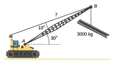
A 12.0m boom, AB, of a crane supporting a 3.00 x 10<sup>3</sup> kg load is shown on the left. The centre of mass of the boom is at its geometric centre, and the mass of the boom is 1.00 x 10<sup>3</sup> kg. Assume the two angles shown are  $10.0^{\circ}$  and  $30.0^{\circ}$ .
