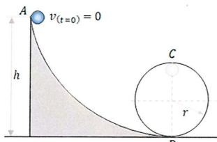
The diagram on the left shows a ball of mass 0.156 kg held h metres above the ground. If h = 1.25m, determine the largest value of the radius, r, that the ball will successfully negotiate the loop without falling off (ie while maintaining circular motion).
